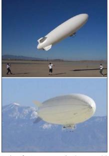
Testing of a Prototype Aerobot is an essential part of the continuing effort to develop an architecture for autonomous operation of aerial vehicles in the atmosphere of Earth as well as of remote planets. These photos show the JPL aerobot during autonomous flight tests conducted at the El Mirage dry lake in the Mojave Desert. The top image shows vehicle liftoff, and the bottom image shows the aerobot in autonomous flight mode.
