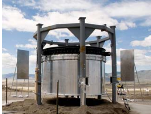
Figure 6. The test of the forward skirt extension's separation system verified the effectiveness of the linear shaped charge and its shock effects.
