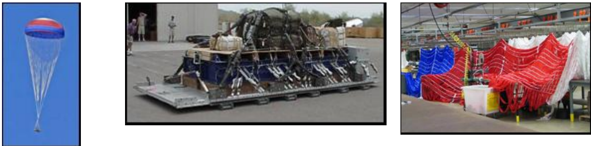
Figure 9. The main parachutes are in the process of fabrication and drop testing.
