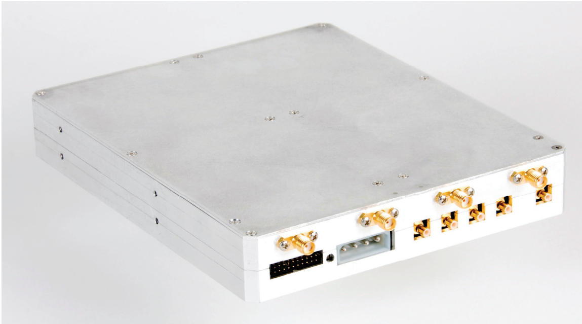
Figure 5. Photo of the SCMT prototype as used for testing. The final four-transceiver system is comprised of two of these units. (NASA photo ED09-0086-10).
