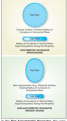
In the Non-Axisymmetric Resonator, the variation of curvature along the periphery in the horizontal plane is chosen such that the ratio between the horizontal and vertical curvatures has the optimum value at some location.
