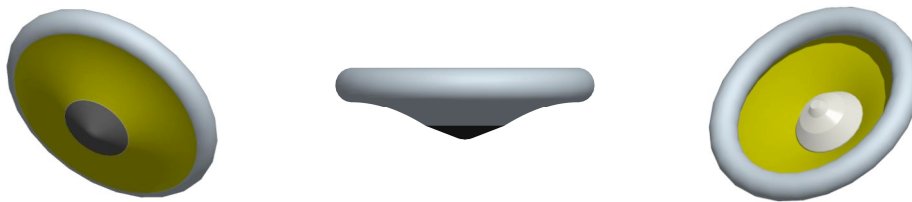
Figure 1. Tension cone inflatable aerodynamic decelerator.
