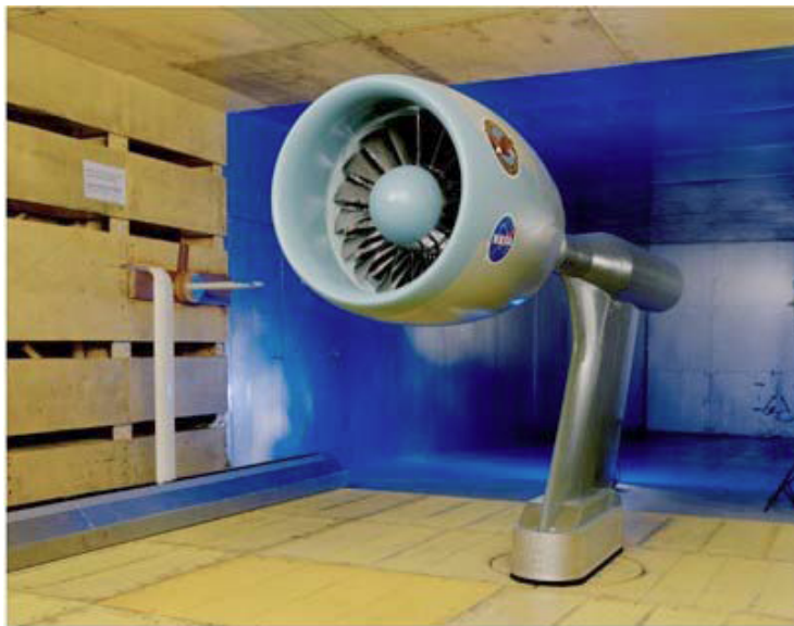
Figure 1: Advanced Ducted Propulsor (ADP) Model Fan 1 installed in the Low Speed Wind Tunnel.
