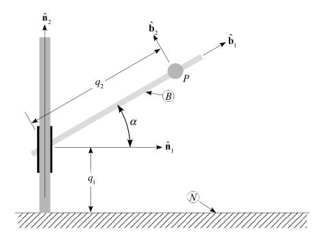
Figure 1: A Particle Moving on a Sliding Inclined Rod
