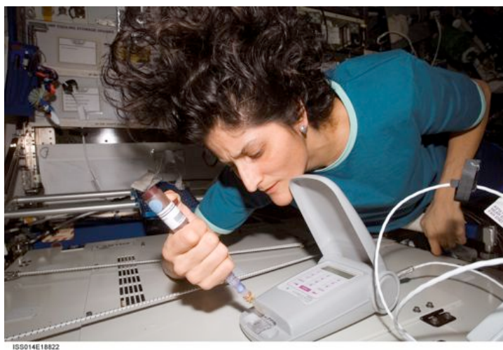
Figure 11. Astronaut Suni Williams dispensing a mixed surface sample during Phase 1 LAL operations (March, 2007)
