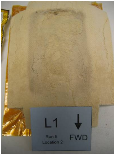
Figure 25. Run 5, Location 2, Layup 1, Pyrogel 6650 post-test.
