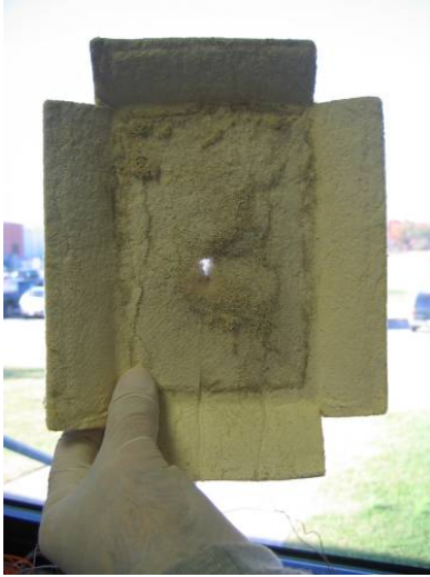
Figure 20. Position 4, Layup 6, Hole in 6650 insulating ply
