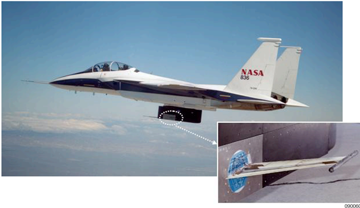
Figure 1. Aerostructures test wing mounted on the NF15B for flight flutter testing.
