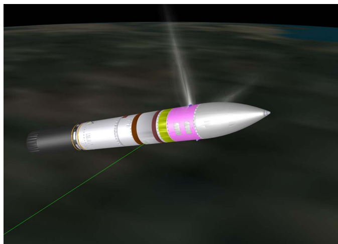
Figure 2. Attitude Control System (ACS) thrusters firing on a 3D detailed model of launch vehicle and payload. Simulation of the thrusters aids in understanding the attitude maneuvers performed. In this figure, the thrusters are turning the vehicle perpendicular to the velocity vector (green line).
