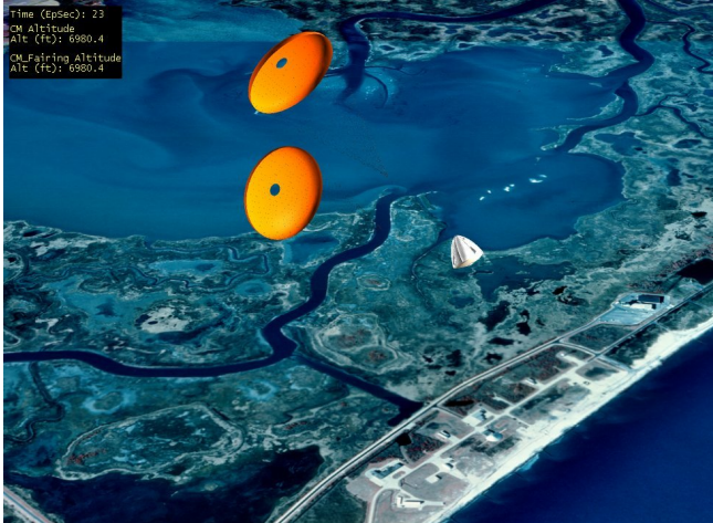
Figure 3. 3D models can show stage separation events, including motor separations, fairing separations, and parachute deployments (seen above).
