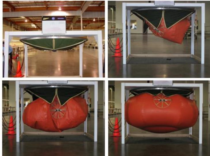
Figure 4: Rapid Inflation Testing
