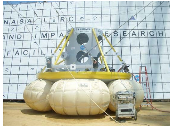
Figure 6. Air bag test article with six air bags
