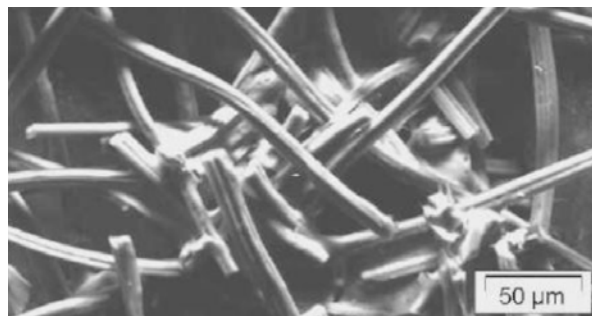
Fig.1. Post-flight scanning electron microscopy micrograph of Stardust TPS surface [Stackpoole, 2008].
