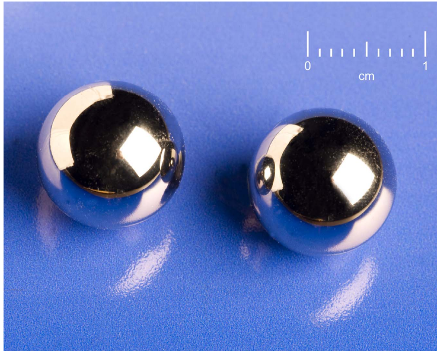
Figure 1.—Photograph of 60NiTi polished ball specimens prior to testing.
