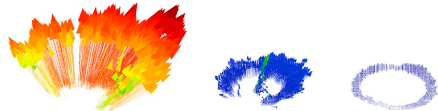
OBLIQUE VIEWS OF THREE-COMPONENT VECTOR PLOTS Oblique impact captured at three different times. Vector colors indicate absolute magnitude of velocity
