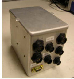
Figure 14.—Linear AC Regulator Controller.
