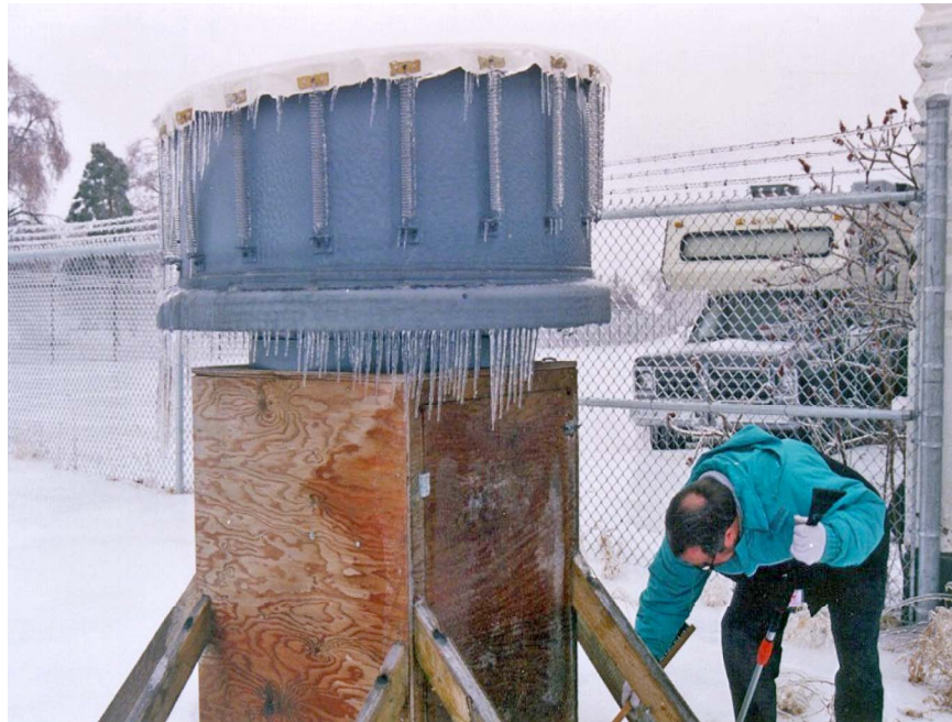
Figure 2.—McGill vertically pointing x-band radar as installed for the AIRS-II field program.
