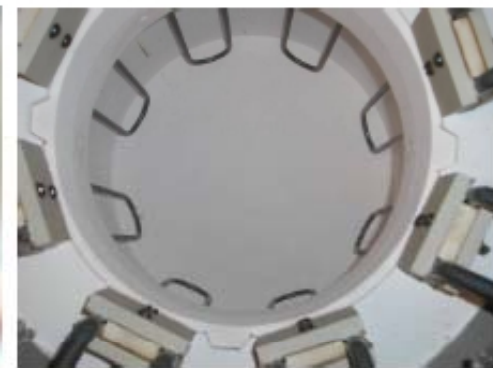
View of the new 10in furnace
