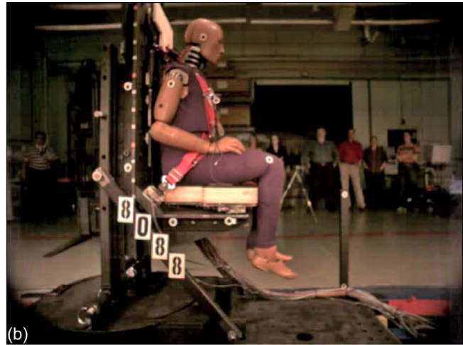
Figure 6.—Sled test with a 10g impulse in the x -direction. Sled motion is to the right. (a) Results. (b) Dummy position.
