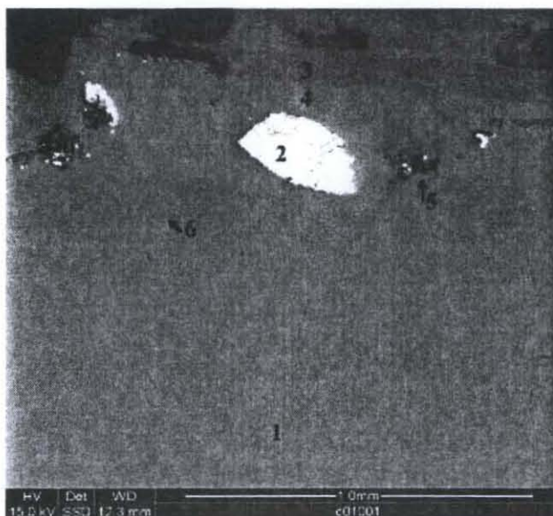
Figure 15. SEM micrograph of sample #14 silicon carbide. Time at temp: 8 hr, atmosphere: air. Marked locations were scanned for composition, results are shown in Table 7. The sample was uncoated.
