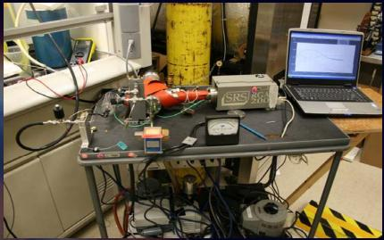
RGA, a small mass spectrometer, was used to analyze gases coming from electrolysis of water. Helium was used as carrier gas and Nitrogen and  $CO_2$  are background gases from air. RGA can also detect degeneration of IL, if present.
