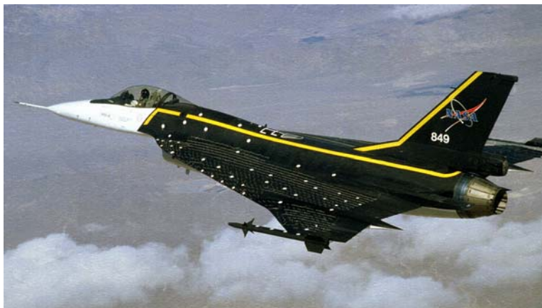
Figure 2. F-16XL-1 aircraft with missiles, tufts, modified flow-visualization paint scheme, and video targets
