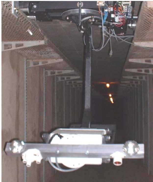
Figure 11. Two ISS-like hemispherical retro-reflectors, OE SRT (bottom left), and 1.5 inch diameter single retro-reflector (bottom right).
