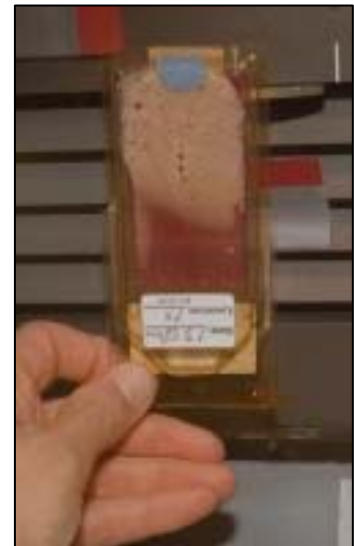
Figure 1. Condensation within a ‘Contact Slide’ onboard ISS
