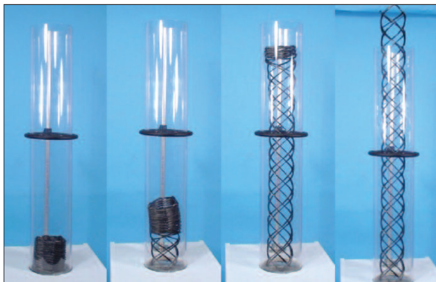
Activation Sequence of an early prototype self-deploying truss shows one one-minute duration from compressed [2.5 in. (6.4 cm)] to deployed [28.5 in. (72.4 cm)].
