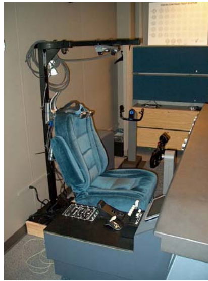
Figure 2. Photo of the head tracker and cockpit set-up.
