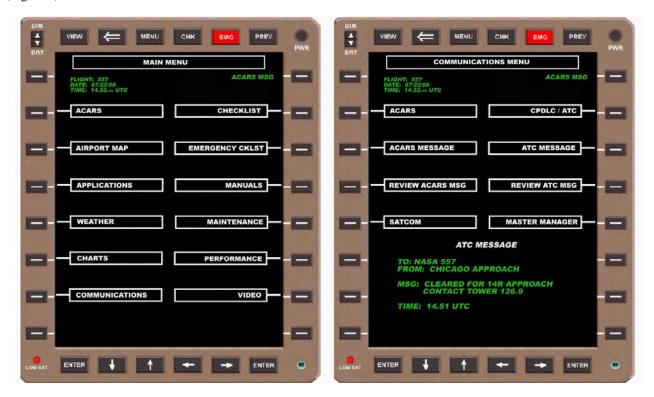
Figure 5. Examples of Electronic Flight Bag (CPDLC) Interface
