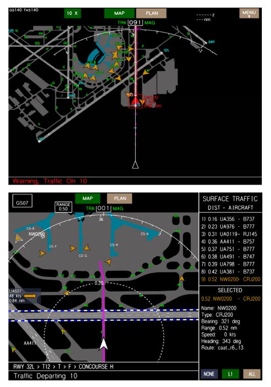
Figure 12. Runway incursion warning alert (left) and active runway occupied primary indication (right)
