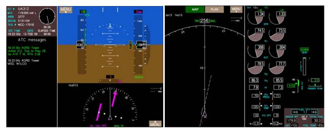
Figure 3. Primary Flight Display and Navigation Display with Half-Screen EICAS
