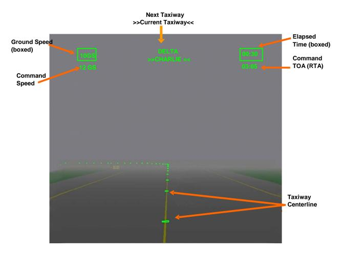
Figure 7. Head-Up Display Symbology for Surface Operations (4DT)
