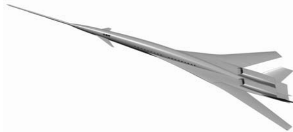
Figure 1. Conceptual low-boom supersonic aircraft configuration.
