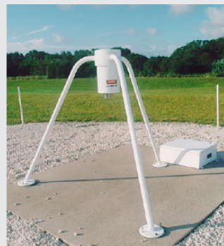
This is one of the 31 electric field mills that compose the Launch Pad Lightning Warning System. They are called mills because they have a rotating, four-bladed shield much like arms of a windmill. The shield contained in the bottom of the round housing alternately exposes and covers metal sensing plates, resulting in an alternating current proportional to the atmospheric electric field.
