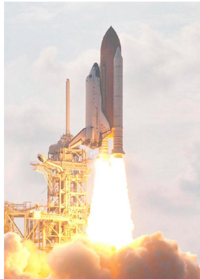
Space Shuttle Endeavour clears the lightning mast and attached catenary wire as it hurtles into space on mission STS-111 to the International Space Station June 5, 2002. The mast and wire provide the primary lightning protection system for the orbiter while it is on the pad. Mission STS-111 is the 18th flight of Endeavour and the 110th flight overall in NASA's space shuttle program.
