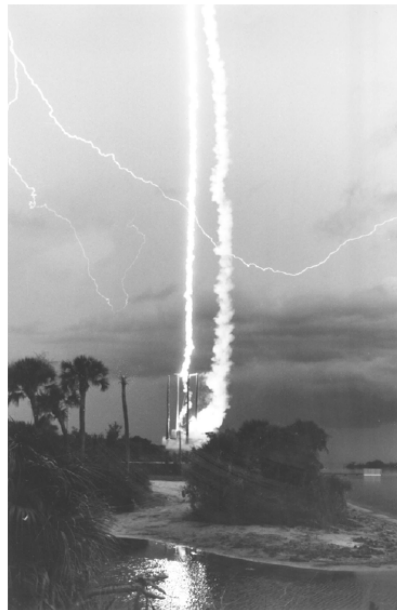
The lightning event begins when lightning strikes the 3,000-foot copper wire being trailed from the 3-foot-tall rocket. The wire is then vaporized as it follows the path to a lightning rod attached to the launcher. As the wire burn dissipates, it creates an effect called "rosary bead lightning." This can be the prelude to natural lightning restrikes. The initiation of a wire burn can also induce natural intercloud lightning during the event, as seen in this sequence.
