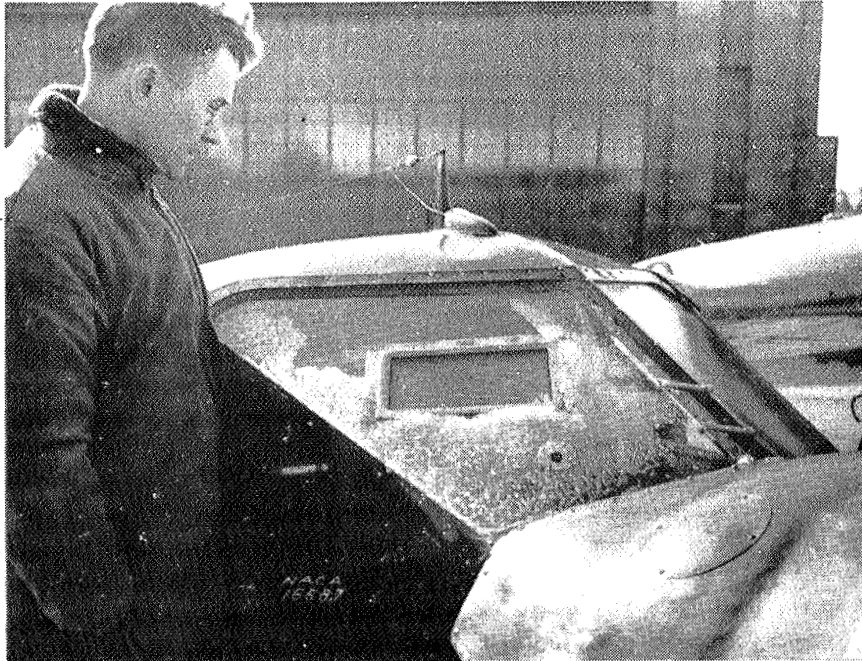
Figure 6.- Ice removal and prevention results illustrated photographically. A large part of the ice on the unprotected region blew away by the air stream during descent.
