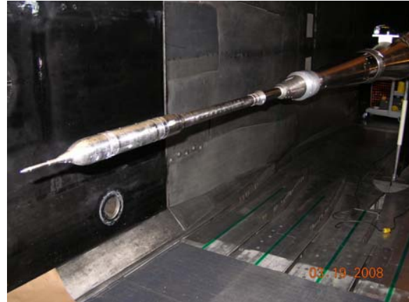
Figure 7. 1% scale pressure model inside the wind tunnel.
