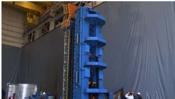
Figure 11. The Ares Projects' Robotic Weld Tool (top) and Vertical Weld Tools (bottom) are now in place to begin testing upper stage manufacturing processes at MSFC.
