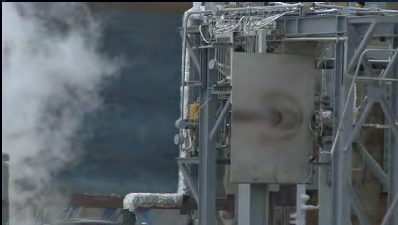
J-2X Workhorse Gas Generator Test Firing Marshall Space Flight Center, AL
