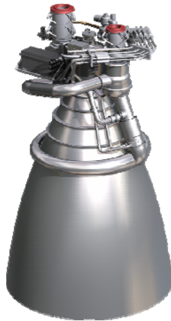
Fig. 14: The J-2X Upper Stage Engine for the Ares I and Ares V.
