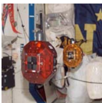
NASA Image: ISS014E17868 - Two satellites fly in formation as part of the Synchronized Position Hold, Engage, Reorient, Experimental Satellites (SPHERES) investigation in the Destiny laboratory module.
