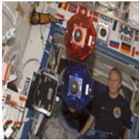
NASA Image: ISS014E08025 - View of the Synchronized Position Hold, Engage, Reorient, Experimental Satellites (SPHERES) floating in the Destiny laboratory module as seen by the Expedition 14 crew. Flight Engineer Thomas Reiter is visible in the background.
