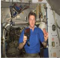
NASA Image: ISS0008E19135 - Expedition 8 Commander Michael Foale holds the SPHERES Ultrasound Beacon and Beacon Tester while performing functionality checks between the Beacon/Beacon Tester and its proximity to a general luminaire assembly in Unity Node 1.
