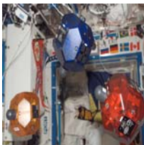
NASA Image: ISS014E17874 - Three satellites fly in formation as part of the Synchronized Position Hold, Engage, Reorient, Experimental Satellites (SPHERES) investigation. This image was taken during Expedition 14 in the Destiny laboratory module.
