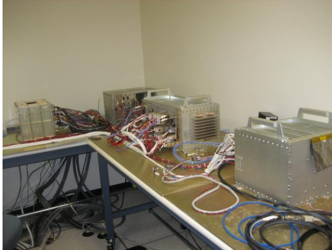
Figure 5.0-2. Solar Dynamics Observatory Flat-Sat Engineering Test Units (left) and Ground Controller (right)
