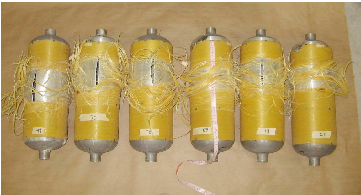
Figure 1: Typical damage of Kevlar COPV bottles that suffered failure.
