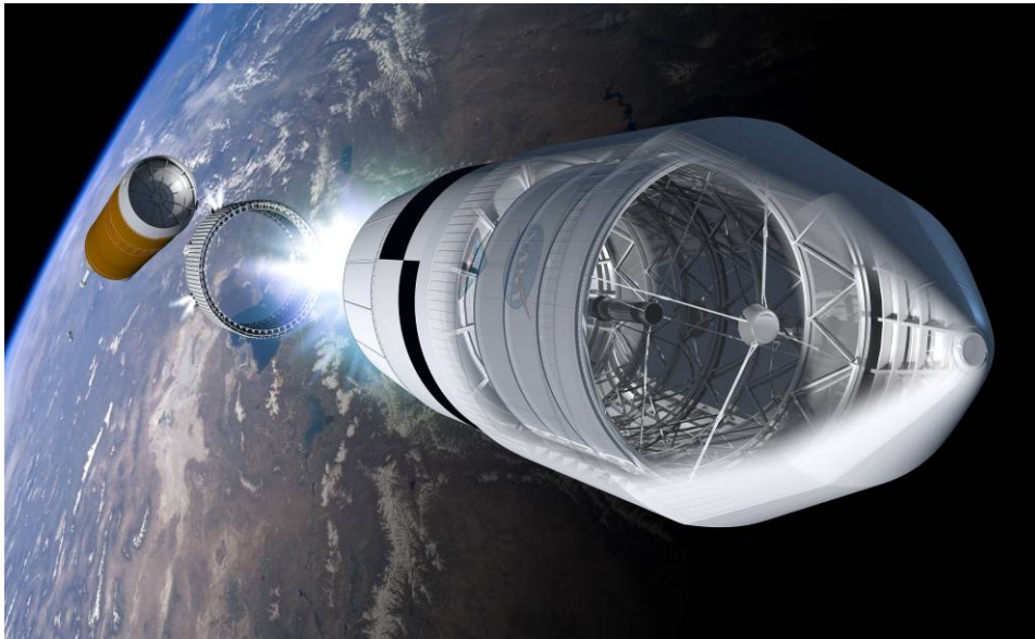
Figure 1 8-meter class monolithic mirror telescope launched in Ares V (Image courtesy of Jack Frassanito & Associates and Harley Thronson)
