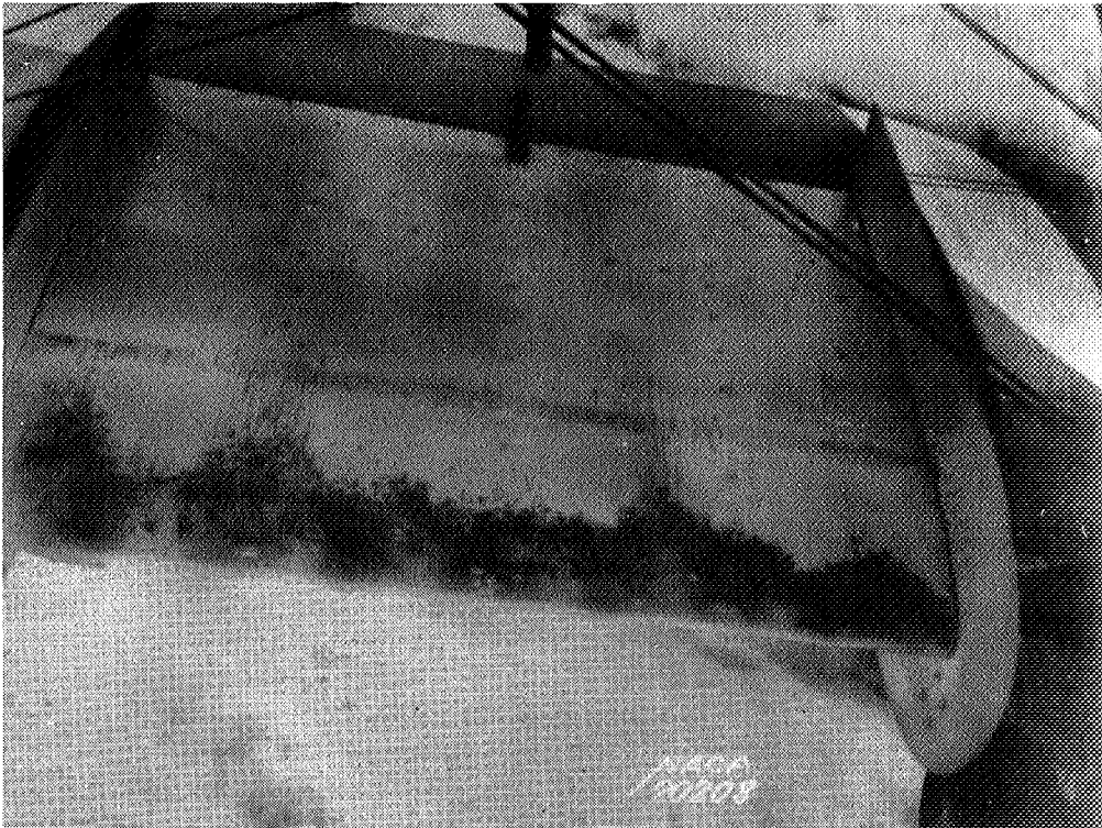
Figure 7.- Nature of ice formation on model wing prior to application of heat.
