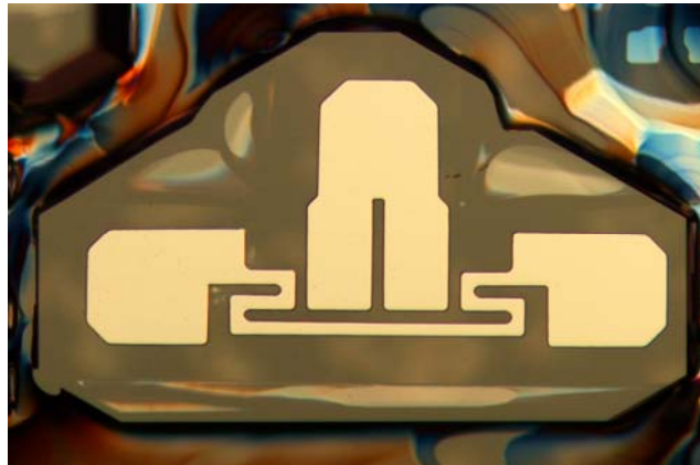
Figure 4. An atomically flat SiC mesa similar to the mesas shown in Figure 3, but now including both the Schottky diode gas sensor and a resistor for temperature control.
