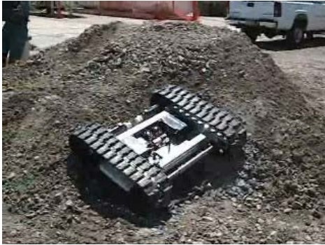
Fig. 10: NASA GRC Sensor Platform “Mule” for demonstrating technologies on the CMU Highlander.
