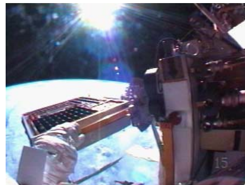
Fig. 3. The FTSCE experiment container being installed on the P6 solar panel strut on the ISS.
