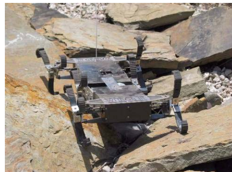
Fig. 9. Whegs™ Vehicle operating in uneven terrain using the locomotion approach of a cockroach (picture courtesy of Case Western Reserve University).
