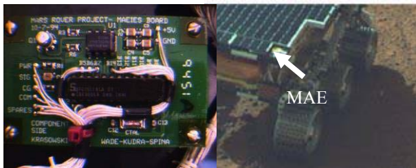
Fig. 1. The MAE circuit board and the location of the MAE on the Pathfinder Sojourner solar panel.
