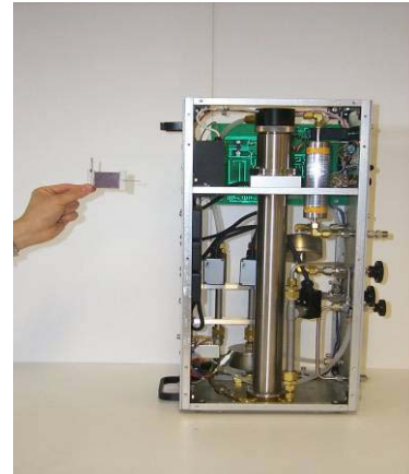
Figure 14. MEMS particulate classifier contrasted with traditional macroscale device.
