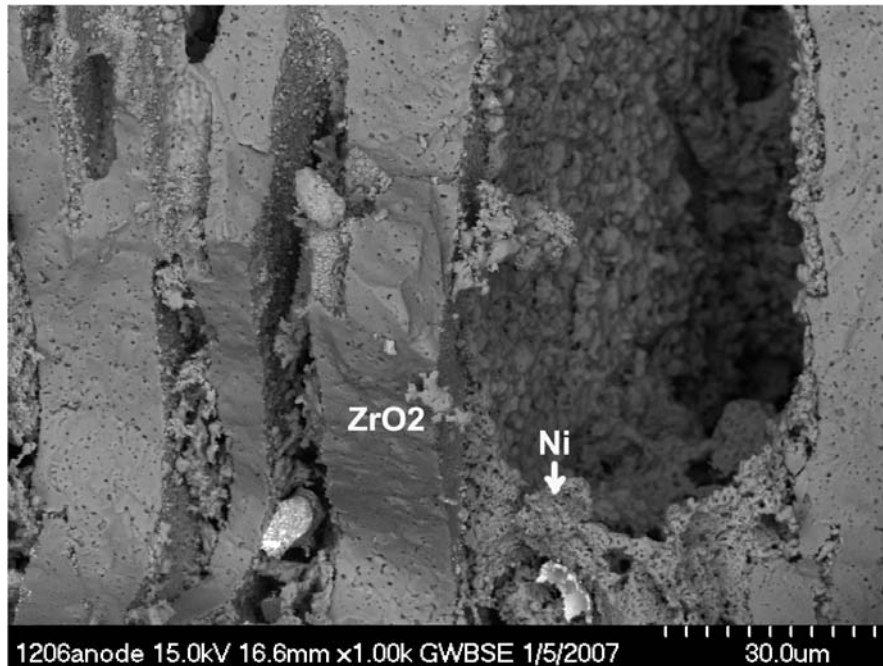
Figure 6: BSC Ni/H 2 -H 2 O electrode, after testing in electrolysis mode. SEM of region adjacent to the electrolyte showing Ni electrode adherent to and complete coverage of YSZ scaffolds.
