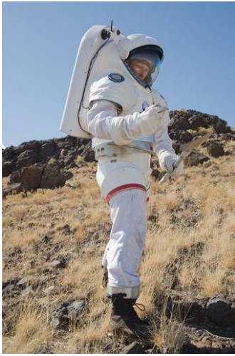
Figure 10 (jsc2008e137994): Mark III Mockup Suit, UPR Configuration
