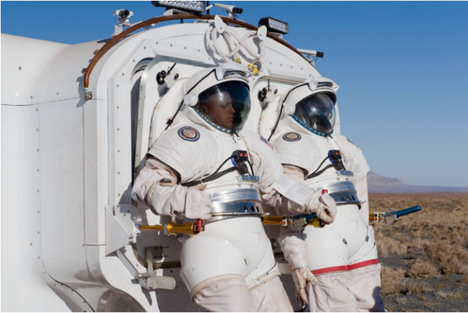
Figure 7 (jsc2008e139052): LER exterior view of aft bulkhead and suit ports with mockup suits attached
