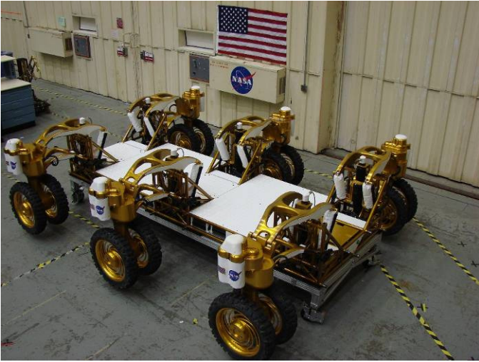
Figure 4: Chariot chassis, or Lunar Truck
