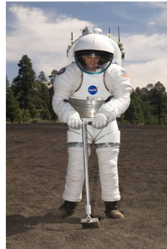
Figure 9 (jsc2007e049514): Mark III Advanced Space Suit Technology Demonstrator
