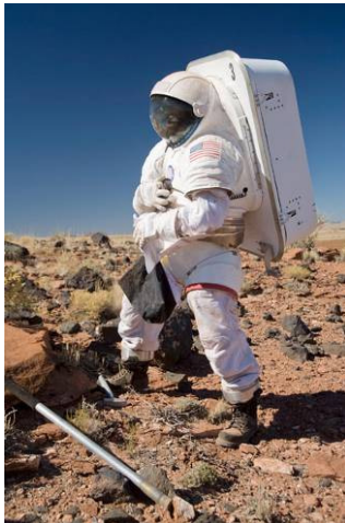
Figure 11 (jsc2008e138835): Mark III Mockup Suits, LER Configuration
