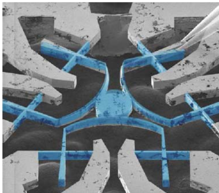
Figure 17: HexFlex manipulator shown in free state (gray) and actuated position (blue). Motion was achieved by pressing on the upper right actuator tab with tweezers (also shown).
