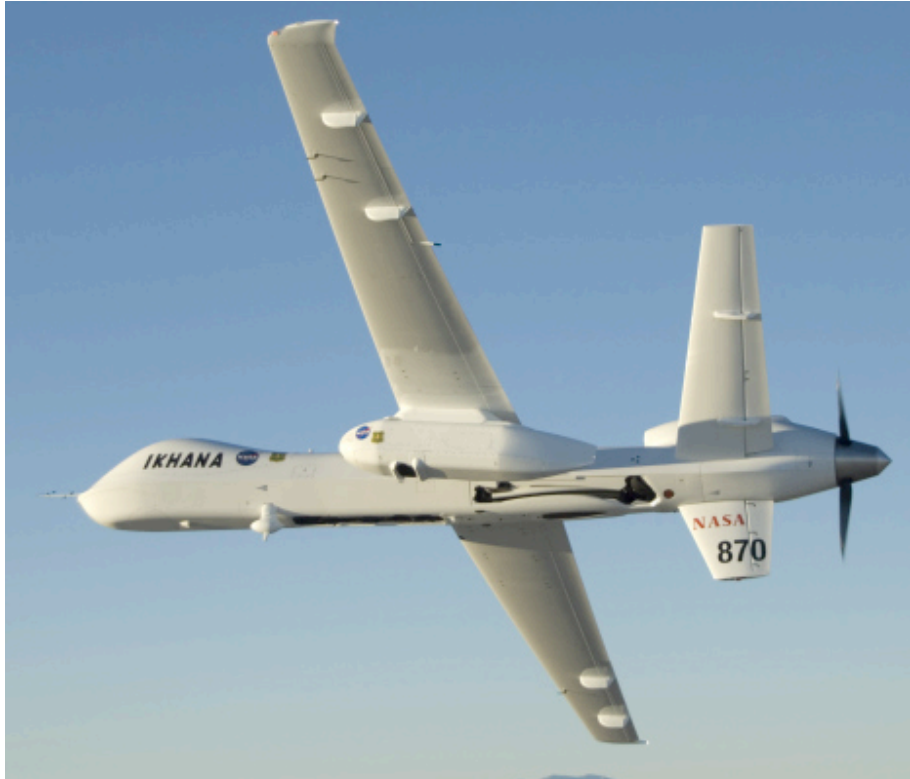
Figure 4. The Ikhana aircraft carrying the fire pod.
