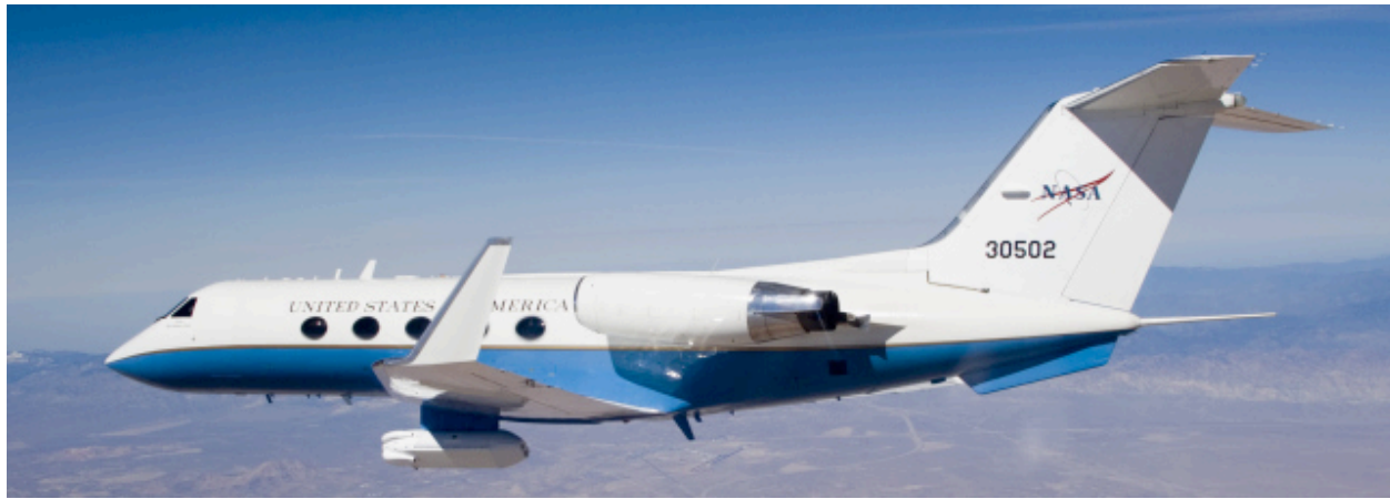
Figure 1. NASA G-III aircraft with synthetic aperture radar pod from NASA Jet Propulsion Laboratory.
