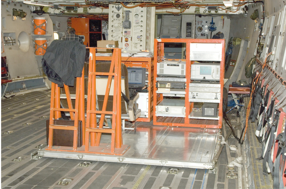
Figure 2. Data rack installed in the C-17 T-1 aircraft.
