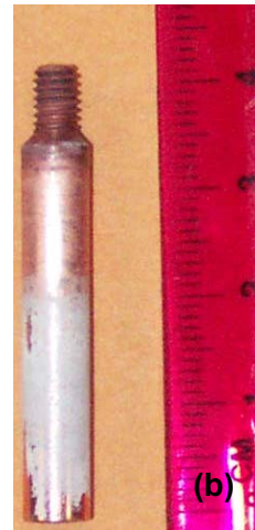
Figure 3. (a) Current density as a function of time for potentiostatic deposition of pure Al using two different electrolyte compositions. (b) Copper electrode with deposited aluminum.
