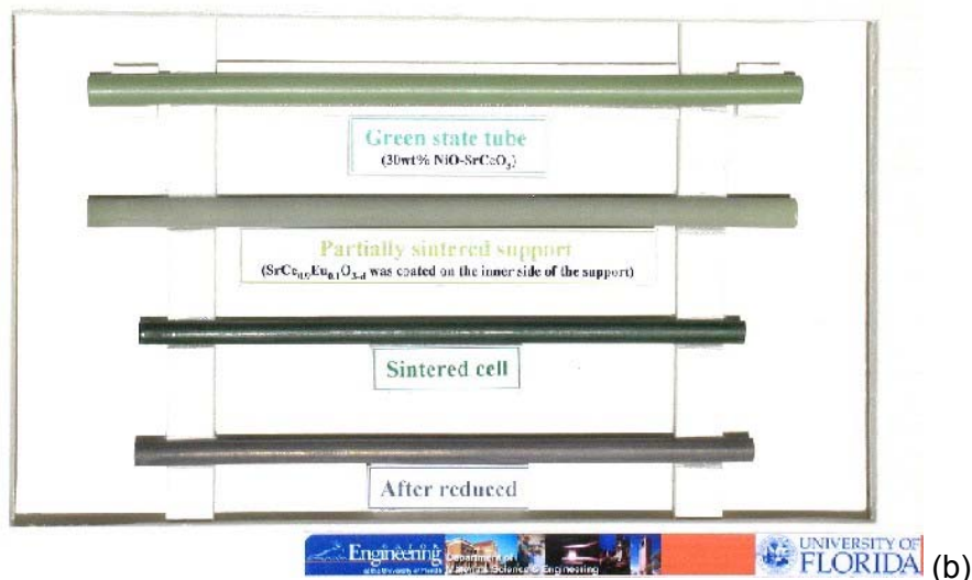
Figure 3. Pictures of (a) tubular hydrogen membrane cells and (b) 10 mol% Eu-doped \text{SrCeO}_3 membrane coated on the inner side of \text{NiO}(\text{Ni})\text{-SrCeO}_3 tubular support at each processing step.
