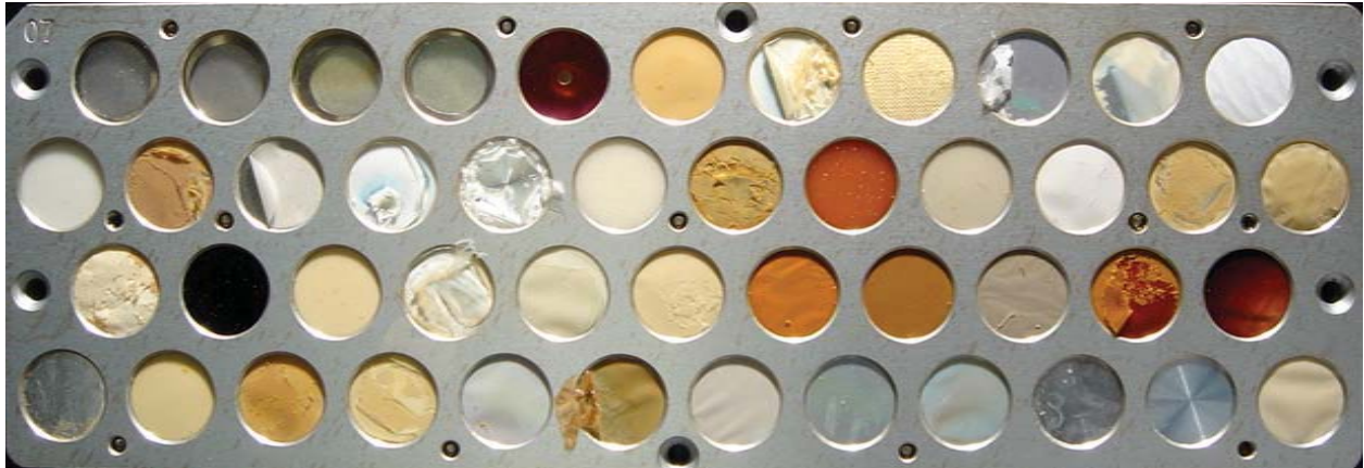
Figure 3.—Photograph of the MISSE 2 PEACE Polymers experiment post-flight.
