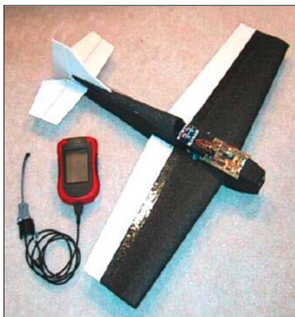
This Model Glider Airplane, instrumented with sensors and control and data-acquisition systems, was used to demonstrate the use of variable-structure control for spin recovery.
