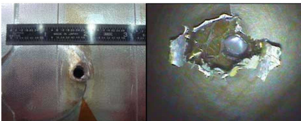
Figure 4. MMOD impacts on STS-118 LH4 radiator.
