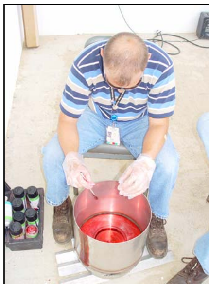
Dye Penetration Testing
