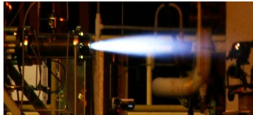
Night firing of MTTP thruster
