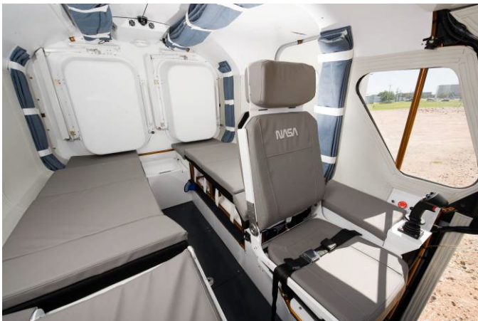
Figure 6. Interior of the SPR showing the left seat and controller. The right seat is in an incline position to illustrate the sleep station. Note the two suit ports in the back.
