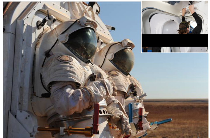
Figure 7. EVA suits locked into the suit ports on the SPR. Insert photo on right shows participant climbing through suit port into suit.
